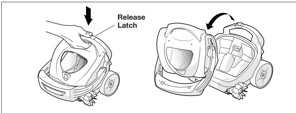
2. Press the filter cover release to remove the filter canister.
