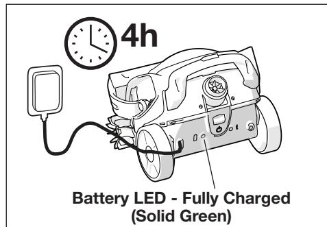
4. When charging is complete, the Battery LED is solid Green, indicating a full charge.
