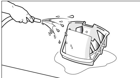
3. Empty debris and rinse the filter canister with fresh water. Reattach canister to the lid.
