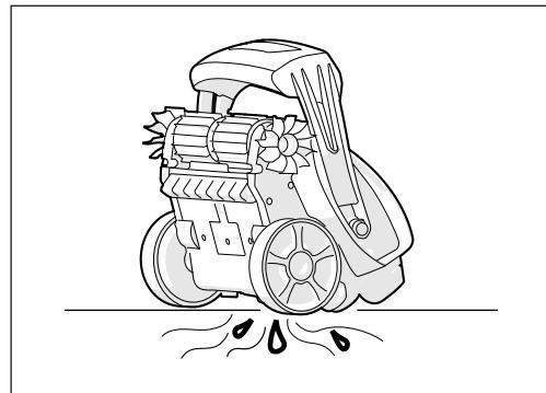
3. Set the cleaner on its back to accelerate water drainage.
